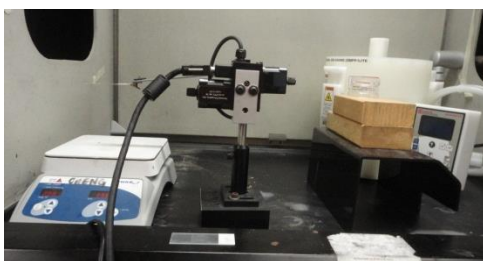
Figure 13: Setup for etching glass slides
