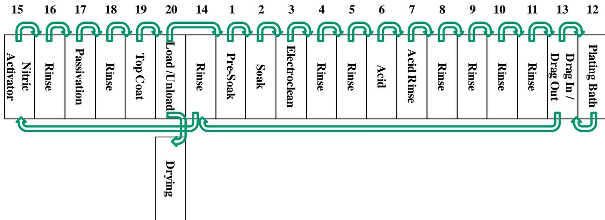
Figure 5.1. Electroplating Process Line Flow Diagram.
