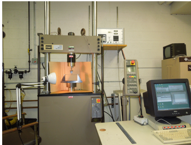
Figure 5.1: Flexural test fixture placed in MTS machine with computerized data recorder and light setup.
