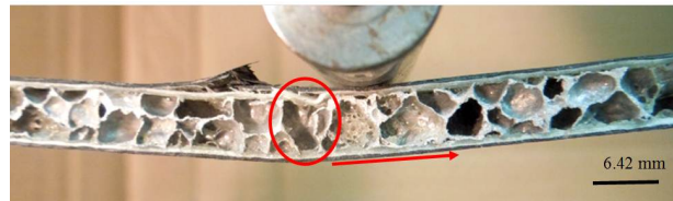
Figure 5.24: Top skin failing.
