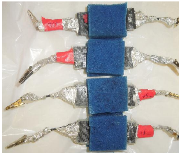
Figure 6.3: Samples covered by foams soaked in NaCl solution for corrosion to take place.
