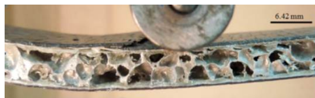
Figure 5.26: Instant width long crack on top skin.
