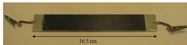
Figure 8.1: Unidirectional carbon fiber/epoxy skin and aluminum core sandwich specimen with electrical connections to measure core resistance.
