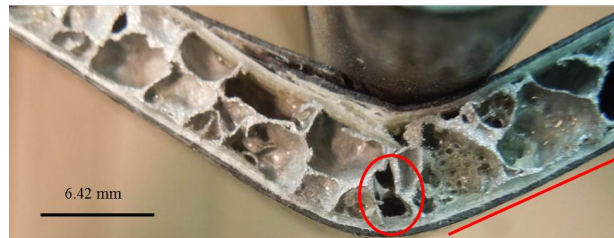
Figure 5.25: Core pore deforming laterally and delamination between different plies of top skin increasing.
