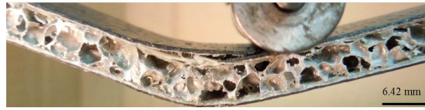
Figure 5.27: Delamination at carbon fabric/epoxy and GFRP interface.
