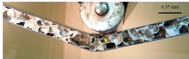
Figure 5.14: Fiber splitting in top skin.
