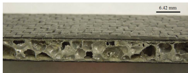
Figure 7.7: Type B unsealed sample after 72 days exposure in room atmosphere.
