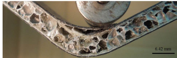
Figure 5.28: Delamination with increased deflection.
