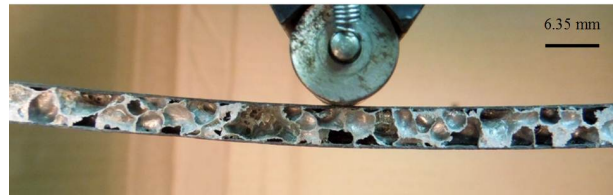
Figure 5.10: Moment just before failure initiates at top skin.
