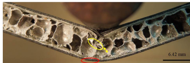
Figure 5.21: Core densification and fiber splitting at bottom skin.
