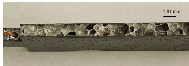
Figure 7.8: Type A unsealed sample after 72 days exposure in room atmosphere.
