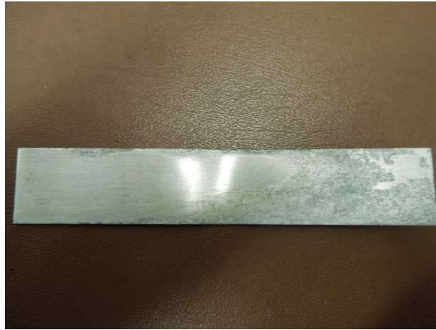
Figure 8.7: Corrosion product on core after removing the skin totally and cleaning the core of above figure.
