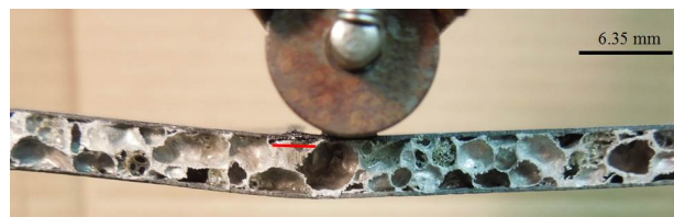
Figure 5.5: Failure initiated in top skin.
