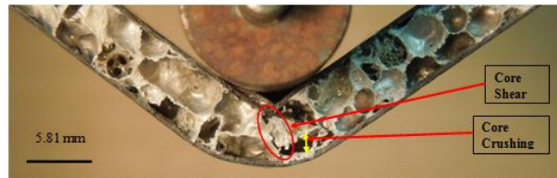
Figure 5.9: Core shear with further core crushing.
