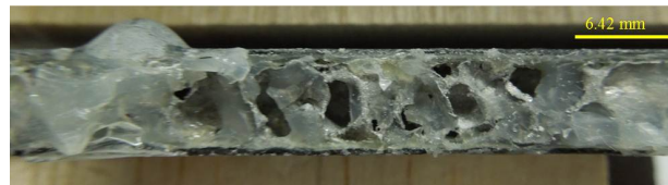
Figure 7.16: Peeled core of sealed type B sample.
