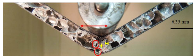
Figure 5.16: With increased deflection core crushing and top skin delamination increases.
