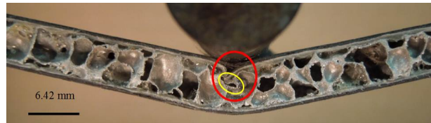
Figure 5.20: Failure in the carbon fabric/epoxy plies of top skin and core crushing continuing.
