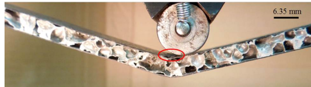
Figure 5.13: Cracked top skin parts overlapping each other.
