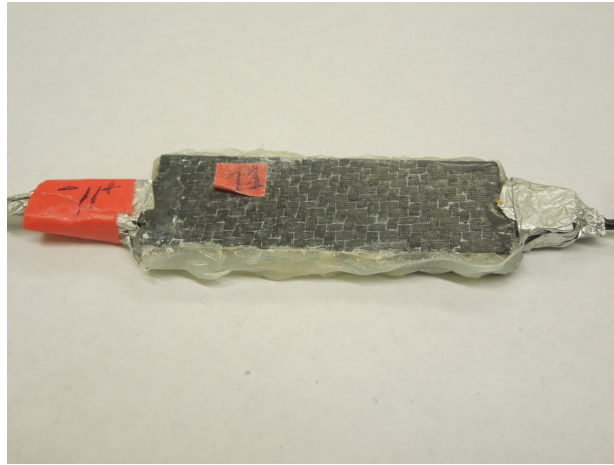
Figure 4.10: Exposed parts of the sandwich beam sealed using silicon chalk and ends covered by aluminum foil with epoxy layers on top.
