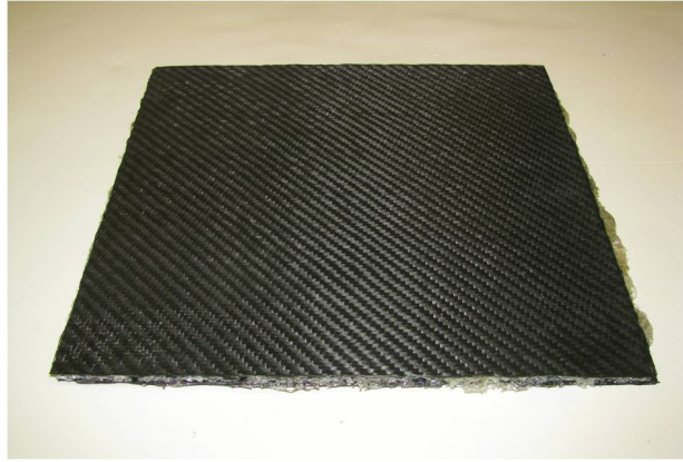
Figure 4.5: Cured carbon fabric/epoxy- aluminum foam sandwich panel.
