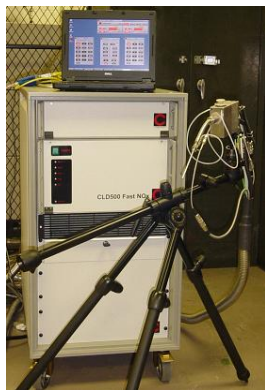
Figure 3.3 Fast NO analyzer (CLD500) provided by Cambustion [66].
