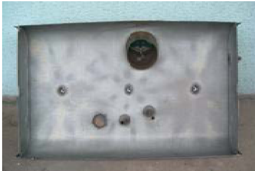
Figure 1 Upper half of fuel tank
