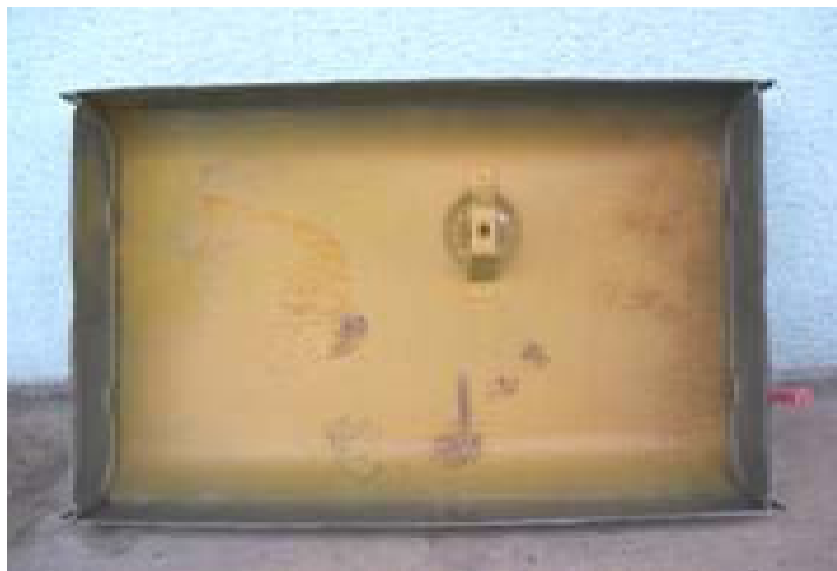
Figure 2 Lower half of fuel tank
