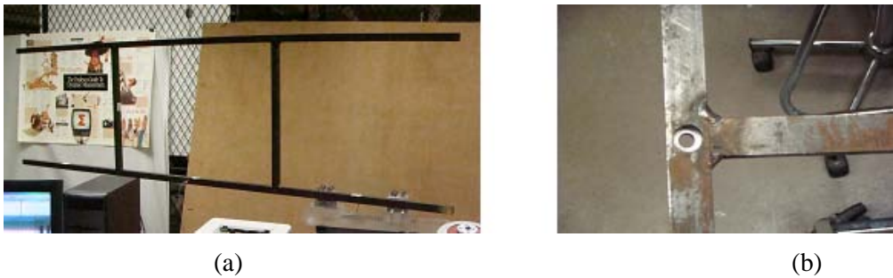
Figure 3.5 A ladder shaped frame for testing: (a) the whole shape; (b) a typical 2-D joint
