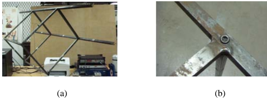
Figure 3.7 A combo beam assembly for testing: (a) the whole shape; (b) a screw joint
