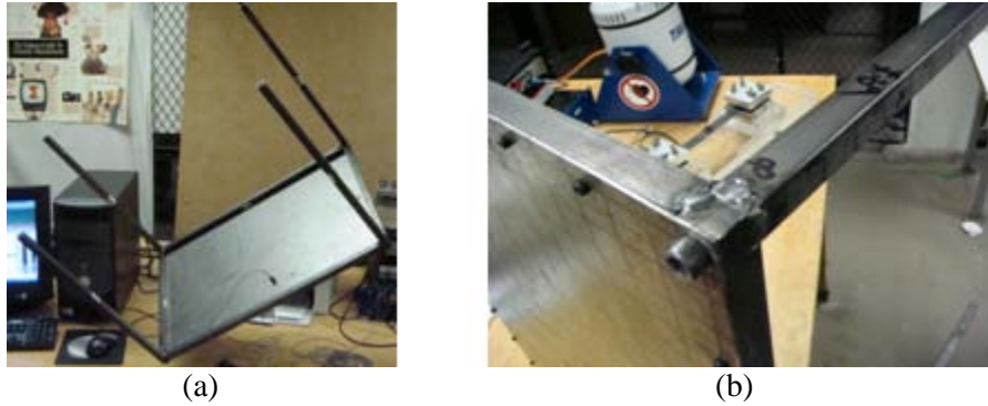
Figure 5.6 A test beam-plate structure: (a) the whole shape; (b) a typical plate-beam junction
