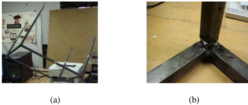
Figure 3.6 A table shaped 3-D frame for testing: (a) the whole shape; (b) a typical 3-D joint
