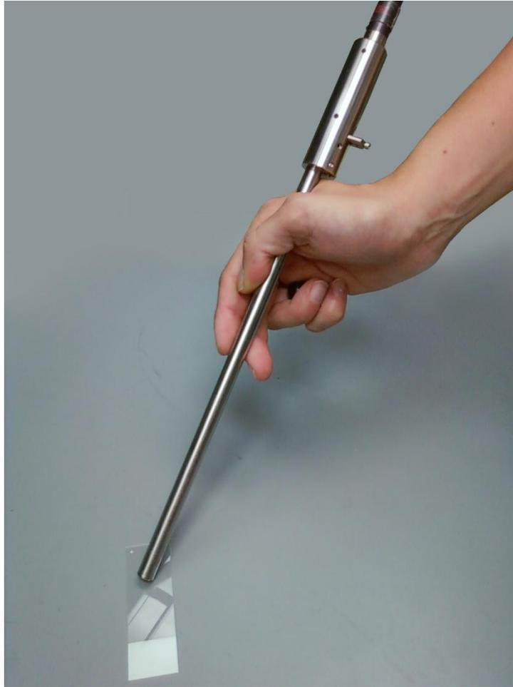
**Figure 3-3: Raman spectroscopy probe**
