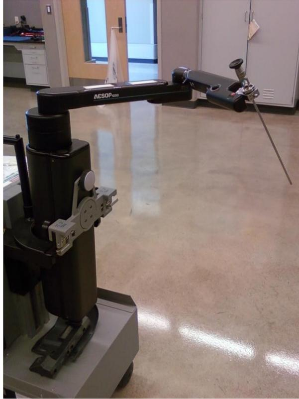
Figure 5-1: AESOP 1000 robotic arm
