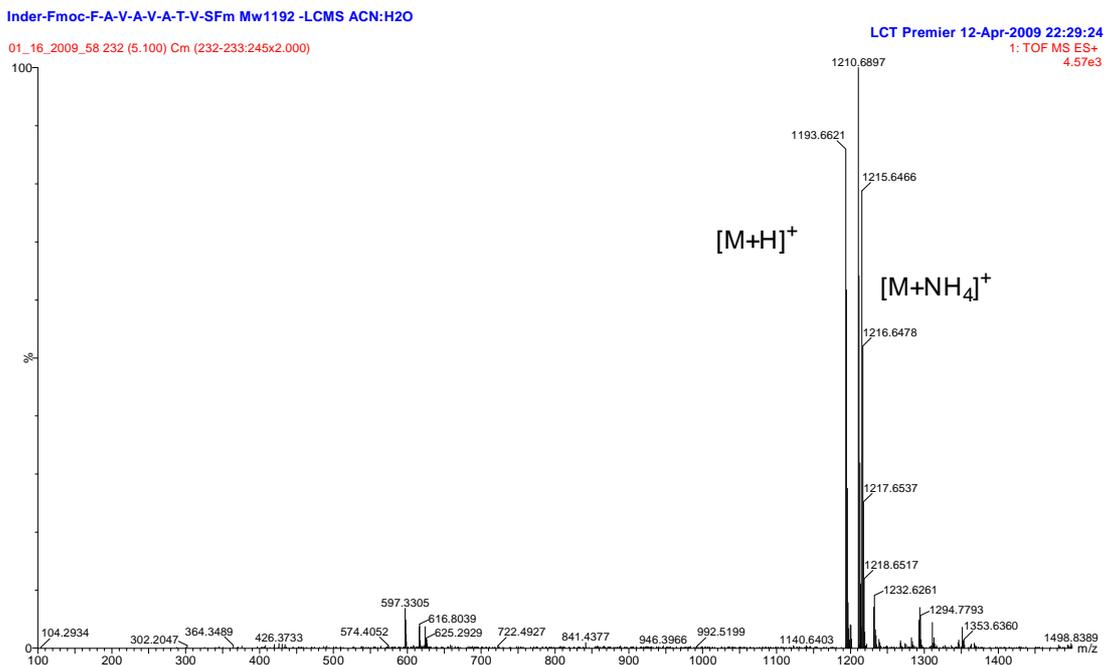
**Figure 34. ESI-MS spectrum of the peak eluting at 11.66 min [Fmoc-L-Phe-L-Ala-L-Val-L-Ala-L-Val-L-Ala-L-Thr-L-Val-SFm (215)]**
