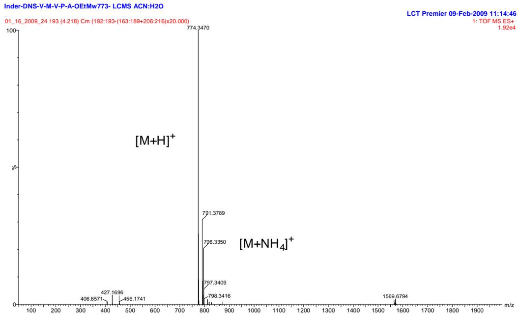
Figure 21. ESI-HRMS spectrum of the peak eluting at 4.22 min [DNS-L-Val-L-Met-L-Val-L-Pro-L-Ala-OEt (174)]
