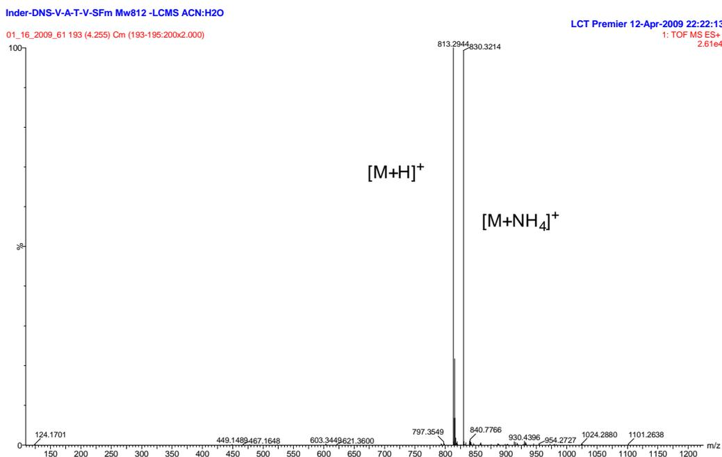
**Figure 25. ESI-HRMS spectrum of the peak eluting at 4.27 min [DNS-L-Val-L-Ala-L-Thr-L-Val-SFm (178)]**
