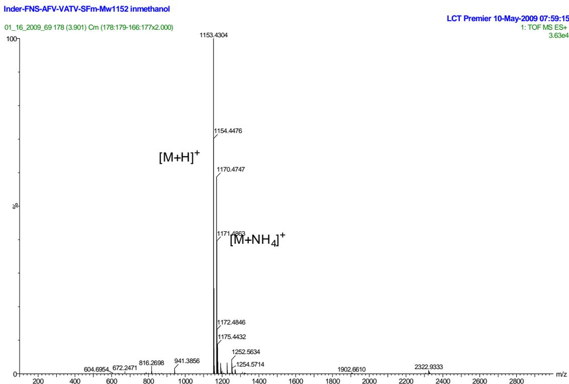
**Figure 32. ESI-HRMS spectrum of the peak eluting at 10.264 min [FNS-L-Ala-L-Phe-L-Val-L-Val-L-Ala-L-Thr-L-Val-SFm (210)]**
