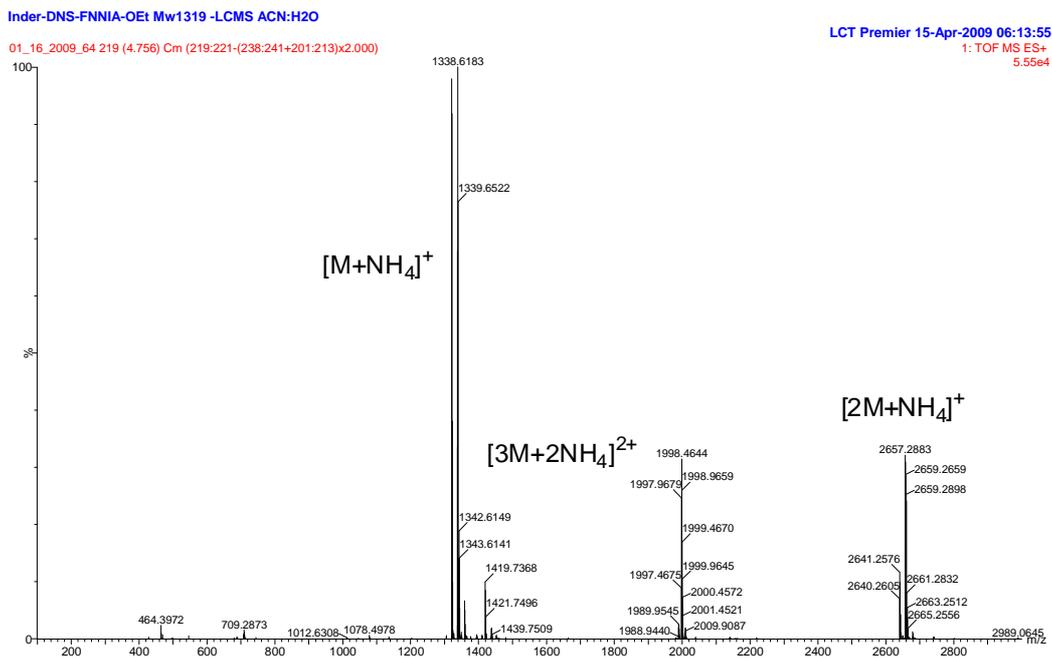
Figure 23. ESI-HRMS spectrum of the peak eluting at 4.76 min [DNS-L-Phe-L-Asn(Trt)-L-Asn(Trt)-L-Ile-L-Ala-OEt (175)]
