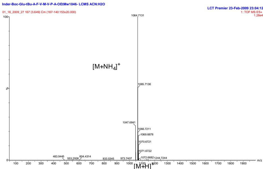
**Figure 29. ESI-HRMS spectrum of the peak eluting at 3.58 min (Boc-L-Glu(L-Ala-L-Phe-L-Val-L-Met-L-Val-L-Pro-L-Ala-OEt)-OtBu)**
