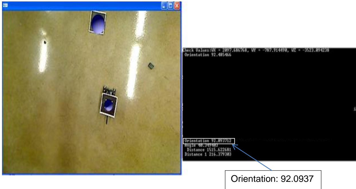
Figure 27: Representation of Orientation of Robot with respect to Reference Marker.
