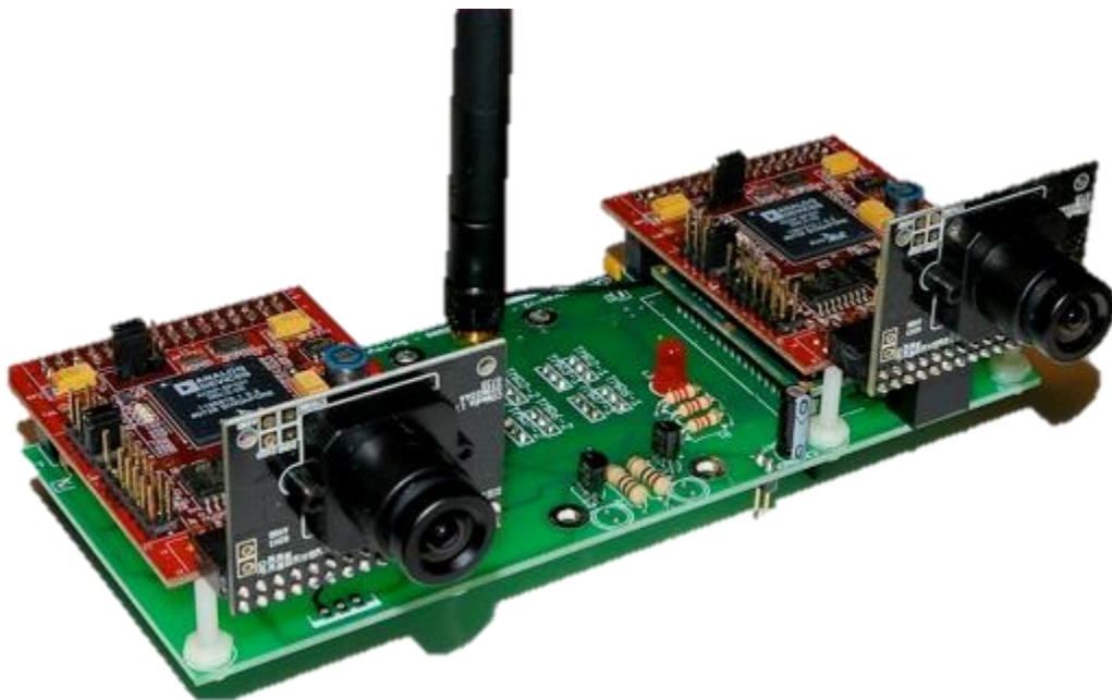
Figure 46: Stereo Vision system for SRV-1 [19].
