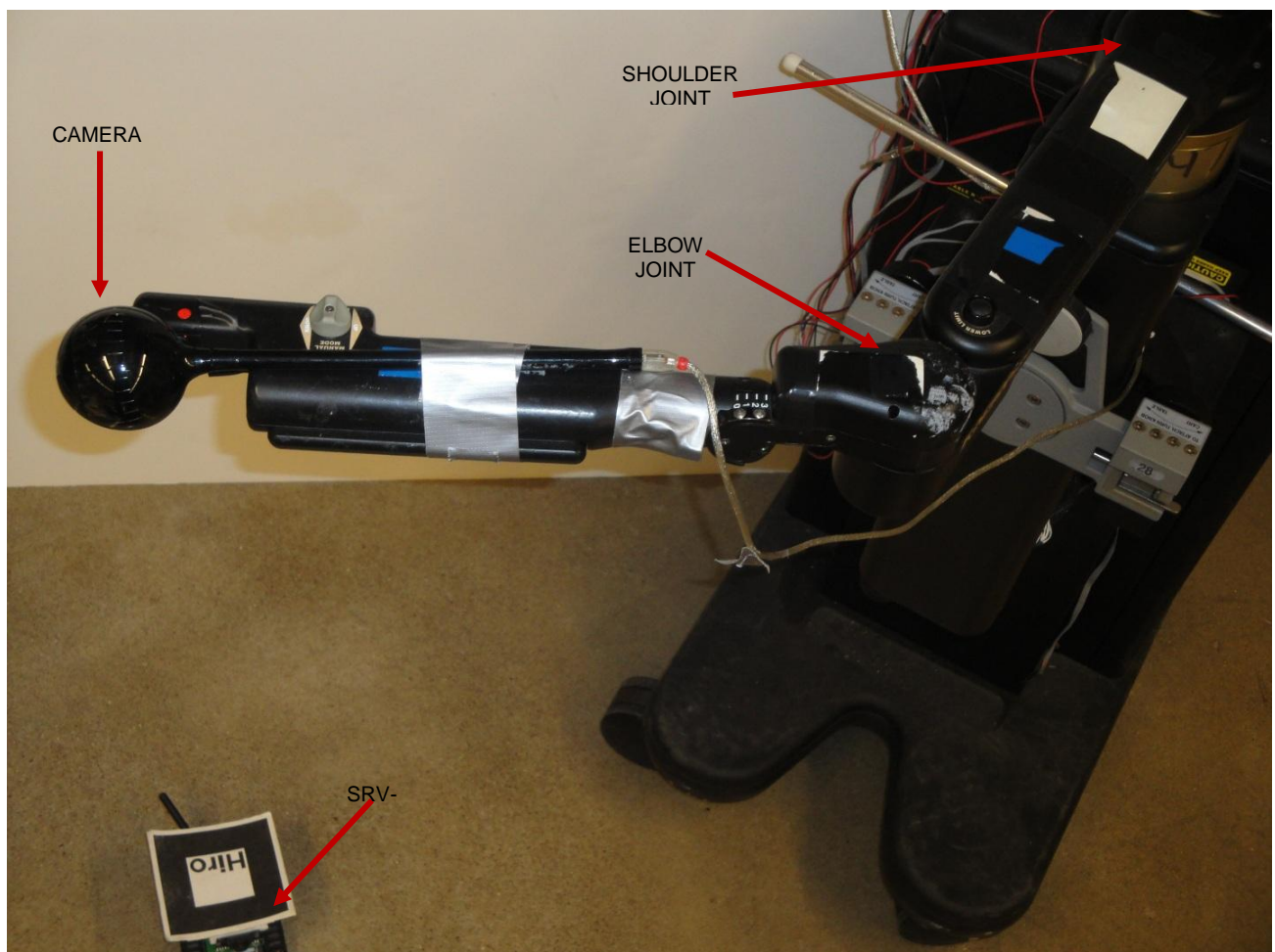
Figure 11: Here, the camera is held by the Aesop arm, and it tracks a ground robot pattern.
