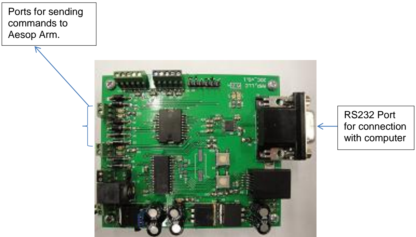
Figure 12: Custom built Motion Control Board for sending command to AESOP arm [17].
