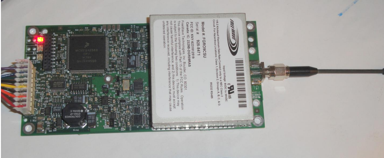
Figure 19: FreeWave 900 MHz board radio with its interface cable, which is connected to the serial to USB connector, connecting the USB serial of the computer.
