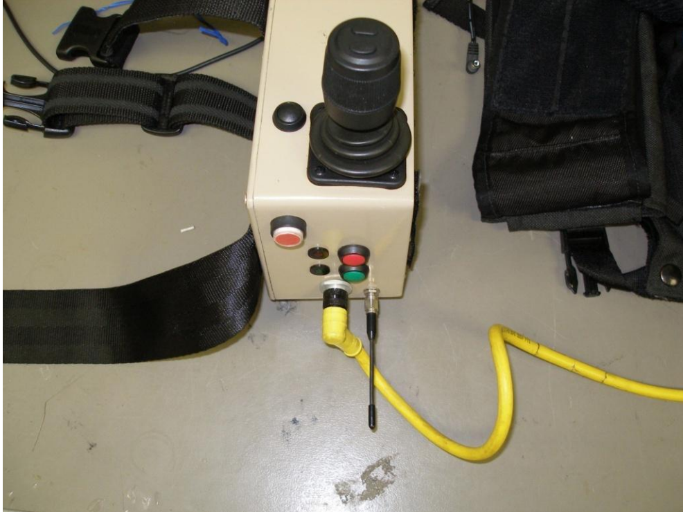
Figure 18: The conventional three degree-of-freedom joystick used to control the ODIS.
