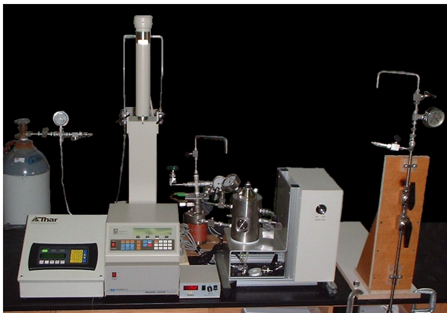
Figure 4. scCO 2 processing reactor, controller and high pressure pump.
