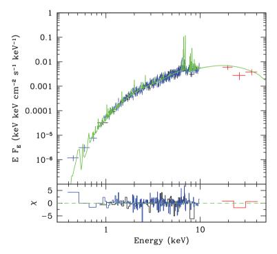
Figure 2. X-ray spectral data from the PN (blue) and MOS1 (black) together with the *INTEGRAL* ISGRI data (red). The best-fitting model comprising a cooling flow, reflection and absorption (see Table 1) is shown in green with residuals to this in the panel below.
