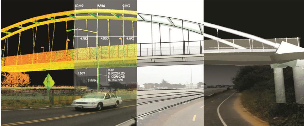
**Figure 20:** Image of bridge showing progression from scanned data on the left, automatic software distance calculations in the left-middle, 3D scan-to-model in the right-middle, and the normal picture of the bridge on the right (Leica Geosystems, 2010).
