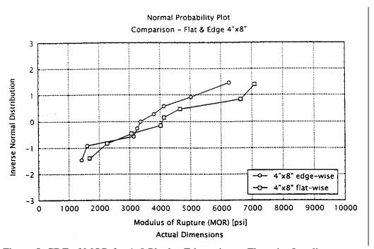
Figure 5. CDF of MOR for 4x8 Planks, Edge-wise vs Flat-wise Loading
