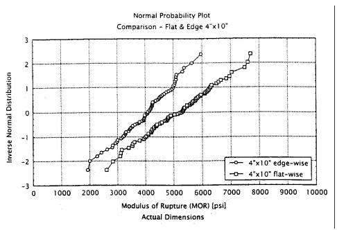
Figure 6. CDF of MOR for 4x10 Planks, Edge-wise vs Flat-wise Loading
