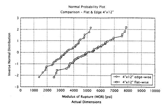
Figure 7. CDF of MOR for 4x12 Planks, Edge-wise vs Flat-wise Loading
